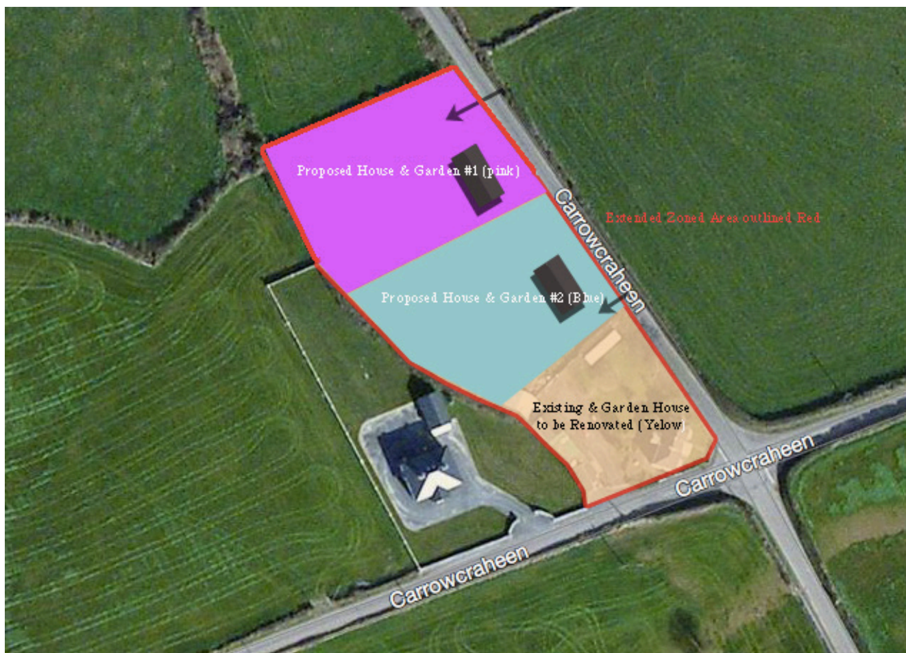
Figure 4 - Aerial Photograph showing proposed site layout for permission to renovate existing dwelling and construct two detached houses. By extending the settlement boundary House #1 can face onto the adjacent public road resulting in a better layout
