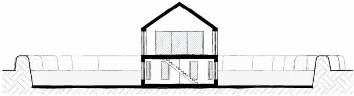
Figure 18.0 Section of proposed scheme. The design is of a unique, high-quality which has been informed by the history and environs of the lands. The dwellings would be provided below the existing floor level resulting in a single-storey appearance.
