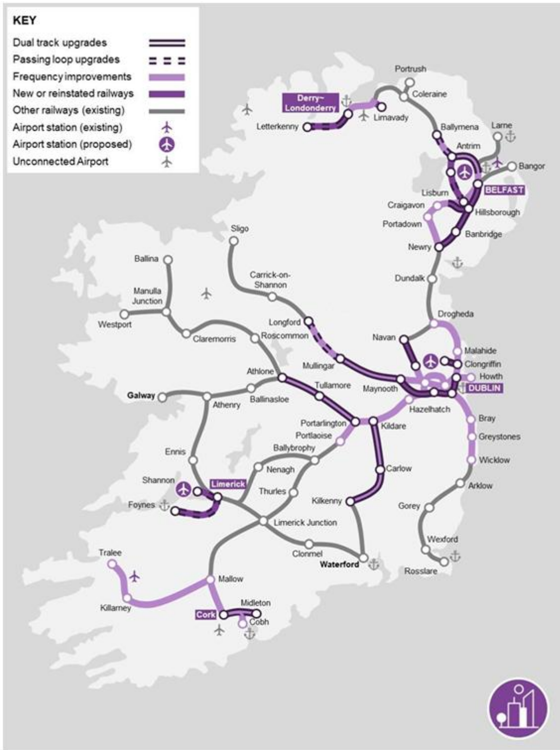
Figure 4: Sustainable Cities and Heavy Rail Interventions (A-ISRR 2024)
